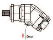
The motor casing flushing can be achieved by means of a flushing valve or directly from the return hose. Too low return pressure must be compensated by a back-pressure valve. The tank hose must be connected into the highest point as shown in the picture.
