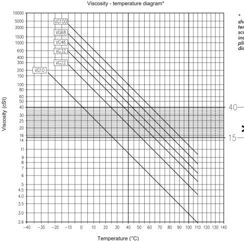
\* The diagram is only an example. It shows the viscosity temperature characterisics of typical fluids with different viscosities but sharing the same viscosity index. Ask to your hydraulic fluid supplier for the real viscosity-temperature diagram of the fluid used in your system. Codice foglio:997-400-24411
